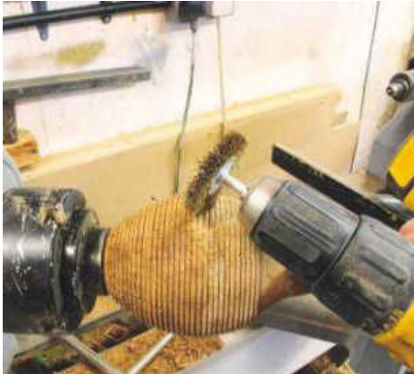
STEP 20. It's time to clean up the beads before we go too thin. The soft brass brush in the drill will smooth up the rough areas. Don't worry if you knock off some of the wood; this just adds texture
